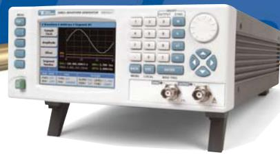
The entire space of the waveform memory is backed up by rechargeable batteries allowing waveforms to be downloaded in the lab and the generator moved to another location for field operation.
